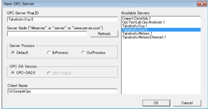
[Server Process] is to select the method of managing the process of OPC Server. When "Default" is selected, it operates initial of OPC Server.
