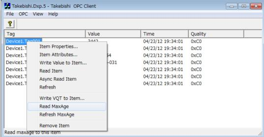
Specify time of "Old" to [MaxAge Value] and execute it. For example, If you specify 1000msec, when the data maintained in the OPC Server is older than 1000msec, the OPC Server acquires the value from device (PLC). And when the data is newer than 1000msec, the OPC Server returns the value of cache (memory of the OPC server).
