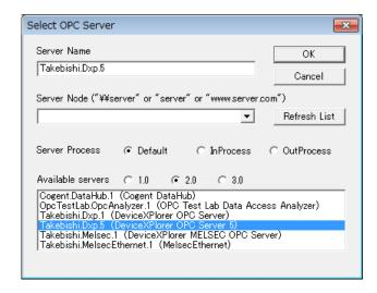
[Server Process] is to select the method of managing the process of OPC Server. When "Default" is selected, it operates initial of OPC Server.
