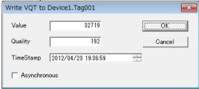
Select "Asynchronous" to execute asynchronously.
