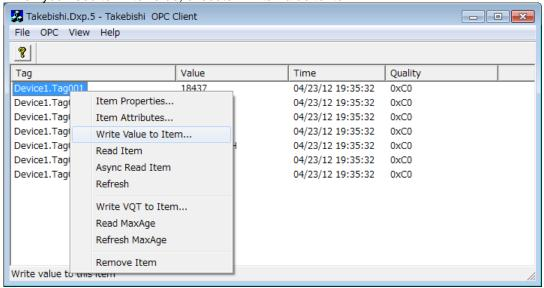
When you write value on array type data, values should be input separated by comma.
