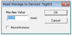
Select "Asynchronous" to execute asynchronously.
